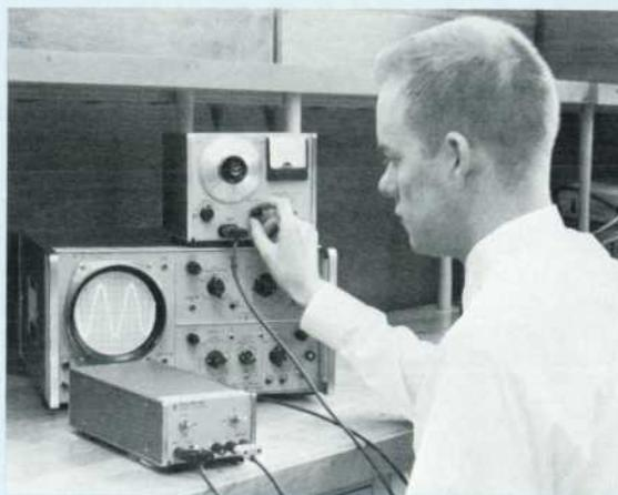
The emitter-follower also drives a second amplifier stage which in turn is followed by an emitter-follower driving a complementary-symmetry output stage. The output impedance of the amplifier is essentially zero ohms and is raised to 50 ohms by a fixed resistor. Following are some typical applications which take advantage of the characteristics of this amplifier.
