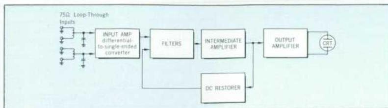
Fig. 4. Block Diagram of Vertical Amplifier in *-hp-* Model 191A Television Waveform Oscilloscope. Passive filters of special design give accurately-shaped responses with high stability. Differential-to-single-ended input amplifier permits use of more stable single-ended filters, has high common mode rejection over wide frequency range.
