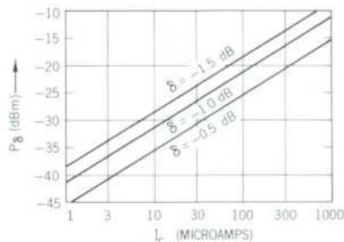
Fig. 6. Upper limit of square-law detection range as a function of bias current for a given square-law error,  $\delta$ .
