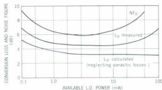
Fig. 6. Conversion loss ( $L_c$ ) and noise figure ( $NF_0$ ) for typical *hpa* 2350 series diodes vs. LO available power.  $f_o = 2$  GHz,  $IF = 30$  MHz,  $NF_{IF} = 1.5$  dB.
