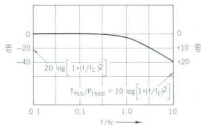
Fig. 7. Normalized frequency response for tangential signal power  $P_{TSS}$  and detected signal current.
