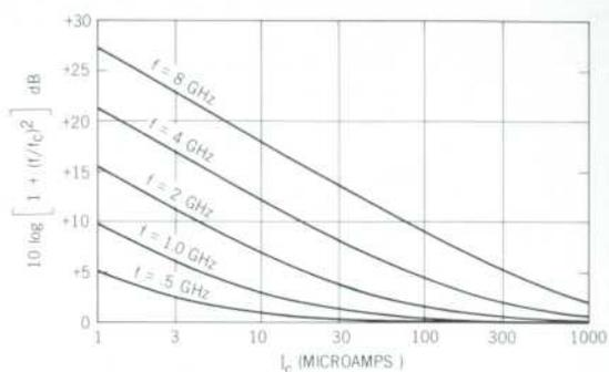
Fig. 4. Variation of tangential sensitivity frequency response correction factor vs. bias current for typical *hpa* 2350 series diodes.
