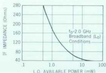
Fig. 10. IF impedance vs. LO available power for typical hpa 2350 series diode.  $IF = 30$  MHz,  $f_0 = 2.0$  GHz, broadband  $L_0$  test conditions.
