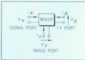
Fig. 1. Representation of mixer as 3-port linear network.
