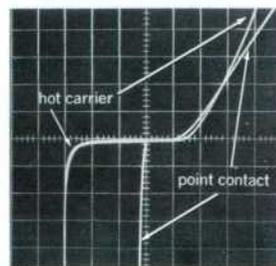
Fig. 7. Double-exposure oscillogram comparing I-V characteristics of typical *hpa* 2350 series diode and point contact diode. Hot carrier diode has steeper forward curve and higher reverse resistance. For forward curves, vertical = 20 mA/div, Horizontal = 0.2 V/div; for reverse, vertical = 10 V/div, horizontal = 10  $\mu$ A/div.
