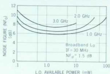
Fig. 9. Noise figure vs. LO available power for a typical hpa 2350 series diode. Broadband  $L_0$ ,  $IF = 30$  MHz,  $NF_{IF} = 1.5$  dB.
