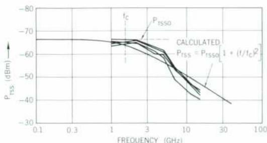
Fig. 8. Measured frequency response of typical hpa 2350 series diodes for tangential signal power  $P_{TSS}$ . Measured at  $27 \mu A$  bias with  $10^3$  Hz video bandwidth.
