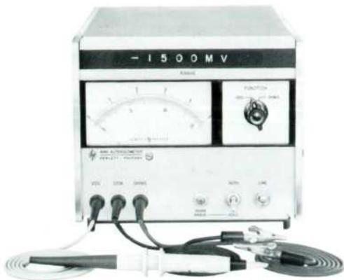
Fig. 2. New *hp* Model 414A Autovoltmeter switches to correct range in less than  $\frac{1}{2}$ -second after contact is made. Illuminated display shows range and selected function (volts or ohms). Mirror-backed, taut-band meter has individually-calibrated scales for high accuracy. Separate probes on 4-ft. cables are provided for voltmeter and ohmmeter functions.
