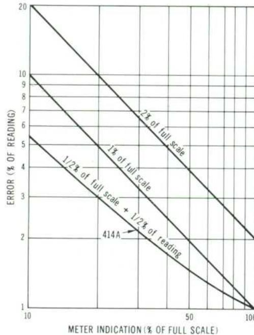
Fig. 1. Accuracy of analog meters as a function of meter deflection. When meter deflection is less than 100% of full scale, *-hp-* Model 414A Autovoltmeter specification of  $\pm\frac{1}{2}\%$  of full scale  $\pm\frac{1}{2}\%$  of reading is more accurate than 1% of full scale specification. Improvement over 2% specification is correspondingly greater.
