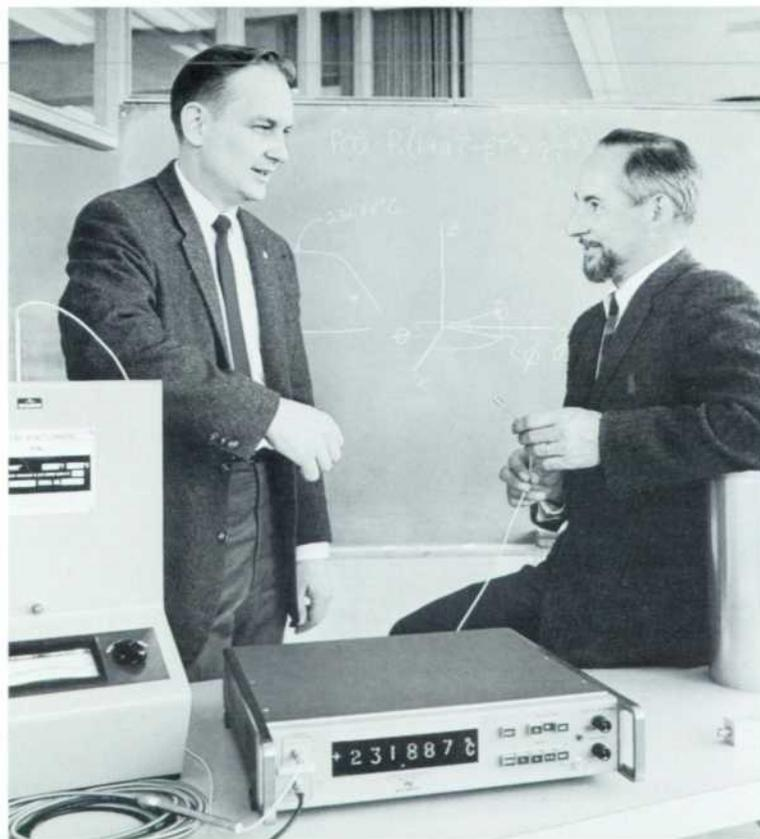
Fig. 1. New linear Quartz Thermometer (foreground) uses quartz resonator as sensor to measure temperatures from  $-40^{\circ}\text{C}$  to  $+230^{\circ}\text{C}$  at resolutions up to  $.0001^{\circ}\text{C}$ . Thermometer can measure temperature at many-meter distances, and digitally-presented data can be recorded and processed by existing hardware. One calibration point of Thermometer is established by freezing-point of tin ( $+231.88^{\circ}\text{C}$ ).
