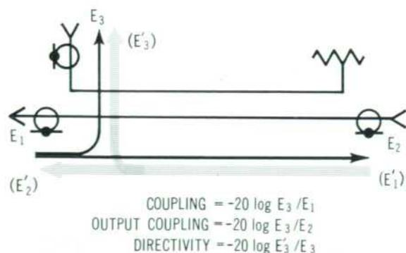
Fig. 4. Definitions of coupling, output coupling, and directivity.  $E_1$  is input voltage,  $E_2$  is voltage out of main arm, and  $E_3$  is voltage out of auxiliary arm.  $E_2'$  and  $E_3'$  are voltages out of input and auxiliary arms respectively with voltage  $E_1$  applied in reverse direction to main arm output. In all specifications, matched loads are considered to be connected to outputs.
