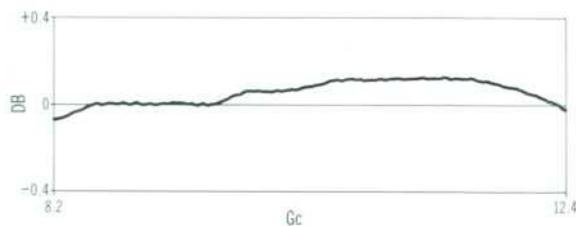
Fig. 3. Net frequency response (curve "a") of two directional couplers in tandem, as in Fig. 2, varies less than  $\pm 0.2$  db by mutual compensation of frequency response curves.
