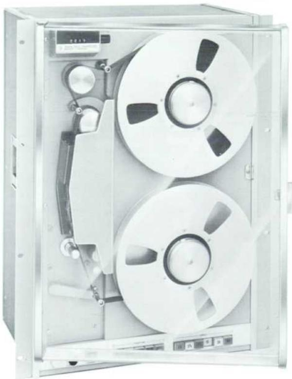
Fig. 1. New magnetic-tape transport designed for use in *-hp-* systems. Transport has mechanical simplicity and a high order of mechanical damping for low long-term flutter. Flutter is less than 0.2% p-p at 60 ips. Tape speed accuracy (average value) is within about 0.1%. Transport complies with IRIG requirements.
