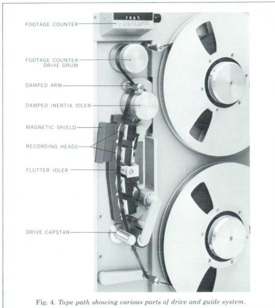
Fig. 4. Tape path showing various parts of drive and guide system.
