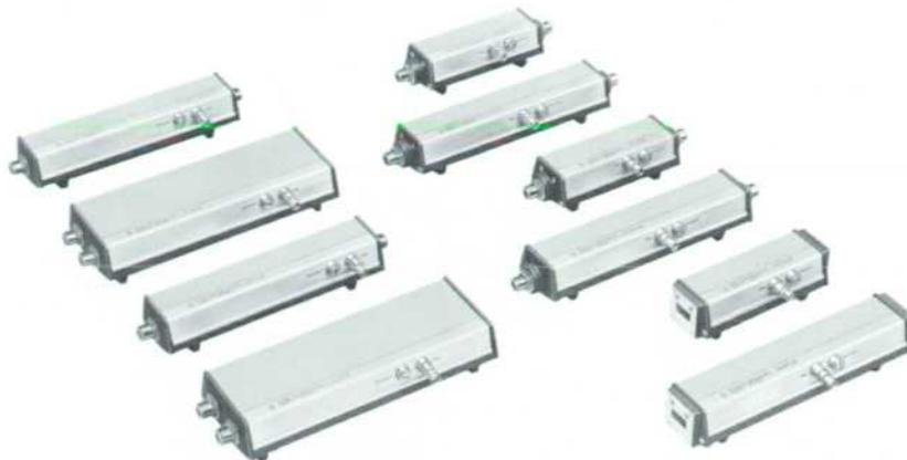
Fig. 13. Family of P-I-N Modulators includes one pair in each frequency range. "A" model of each pair has maximum attenuation range of 35 db, useful for leveling or for amplitude modulation; "B" model has attenuation range of 80 db for pulse or other "on-off" modulation (see Table I).
