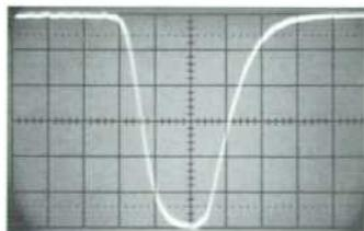
Fig. 2. Pulsed output of new -hp- Model 8614B Signal Source, as demodulated by negative polarity crystal detector, shows fast pulse capabilities. Sweep speed: 0.1  $\mu$ sec/cm; vertical sensitivity: 5 mv/cm; RF frequency: 1350 Mc.
