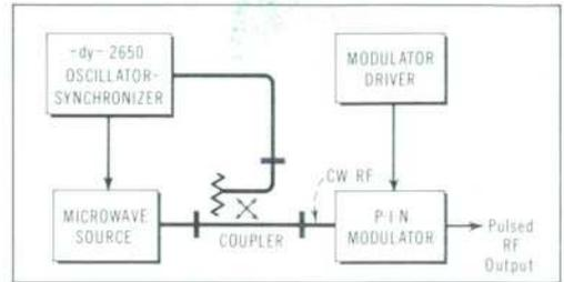
Fig. 4. Highly stable pulsed RF is generated by CW oscillator phase-locked to frequency reference prior to modulation.
