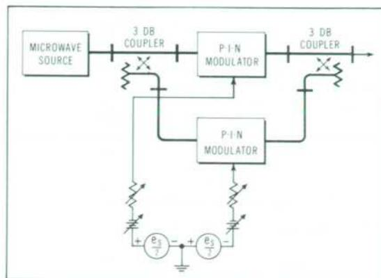
Fig. 7. Two P-I-N Modulators function as balanced modulator by introduction of 180° phase-shift at carrier frequency in one of two parallel RF paths.
