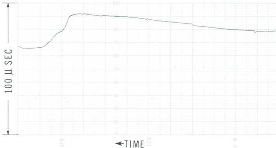
Trace made by Dymec tunable VLF Comparator while checking quartz oscillator against Navy station NBA (24 kc) in Panama (3300-mile path). Chart scale is 100  $\mu$ sec phase difference edge to edge. Slope of 2  $\mu$ sec/hr between 8 A.M. and
