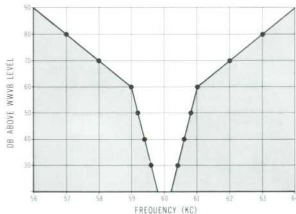
Fig. 13. Interference rejection of *-hp-* Model 117A VLF Comparator. Ordinate represents power level of interfering signal in db above WWVB received signal level. Interference having frequency and amplitude in shaded areas has no effect on operation of VLF Comparator.
