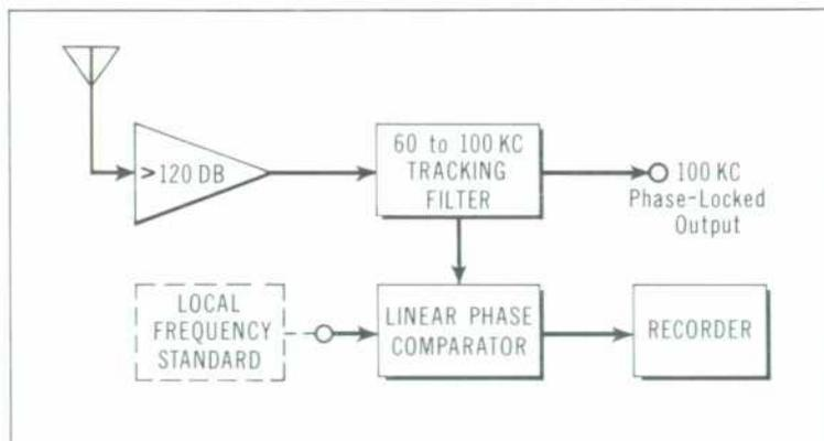
Fig. 4. Simplified diagram of -hp- Model 117A VLF Comparator System. Recorder makes time plot of phase difference between local frequency standard and received standard broadcast carrier.
