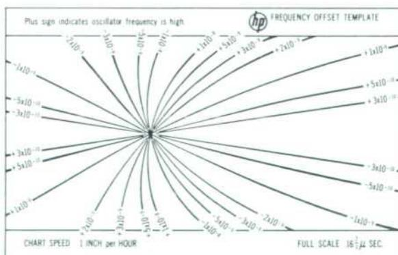
Fig. 6. Transparent template simplifies reading of recorder trace. Template relates slope of trace to frequency offset between local and WWVB signals. Template shown here is for use with  $16\frac{2}{3}$   $\mu$ sec scale (phase difference in microseconds across width of recording). Similar templates are used with 50  $\mu$ sec scale.
