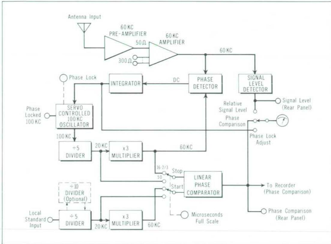
Fig. 5. Block diagram of VLF Comparator System.
