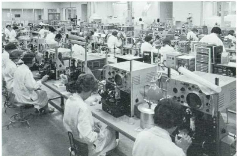
Fig. 4. Assembly area in *-hp-* Associates manufacturing facility. *-hpa-* was established in recent years to produce special semiconductor devices for *-hp-* and for industry.
