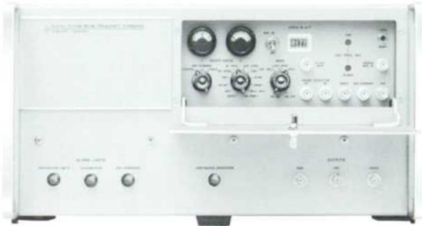
Fig. 7. Front view of Cesium Beam Frequency Standard. Cesium beam standards utilize a quantum-mechanical effect to produce ultra-stable frequencies. Two standards were combined with electronic clocks and power supplies to form an "atomic" clock with stabilities of a few parts in  $10^{12}$ .
