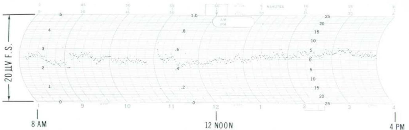
Fig. 5. Graph plots voltage at resistive summation point between +1v and -1v outputs to show stability of standard voltage system during typical working day. Chart scale is  $20 \mu\text{V}$  from edge to edge. System overload trips
