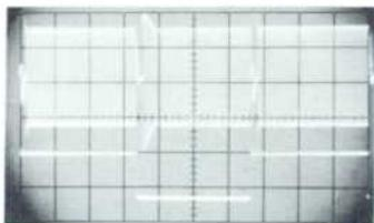
(f) Synthesizer switched between 19.99 Mc and 20 Mc. Sweep is 200  $\mu$ sec/cm.
