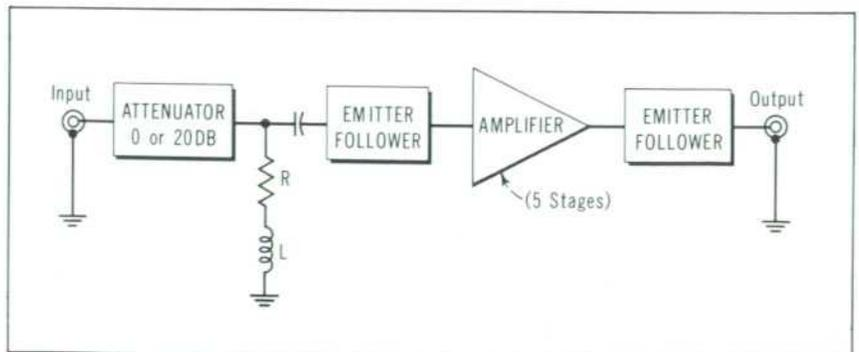
Fig. 5. Elemental block diagram of 461A/462A amplifiers.
