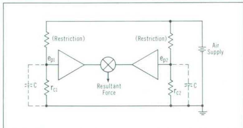
Fig. 8. Electrical analog of one pair of "pads" in multiple-pad bearing of Fig. 7. Capacitances  $C$  are added when air or other compressible fluid is used as lubricant. Voltages  $e_{p1}$  and  $e_{p2}$  represent pressure within pad.
