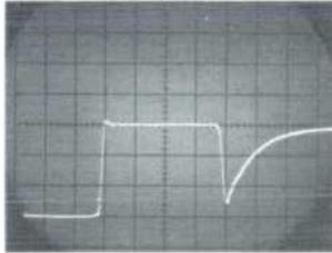
Fig. 17. Reflection from 100 picofarads shunting a 50-ohm line. Sweep speed 2.5 ns/cm. Time constant is  $CZ_0/2$  or 2.5 nanoseconds. The finite rise time prevents the voltage from dropping quite to zero.
