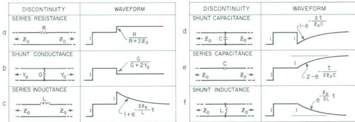
Fig. 6. Typical reflections produced by simple discontinuities.
