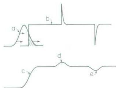
Fig. 7. As the reversed system impulse response (a) scans the ideal curve (b) the integral of the product (shaded area) produces the actual response shown in the lower curve.
