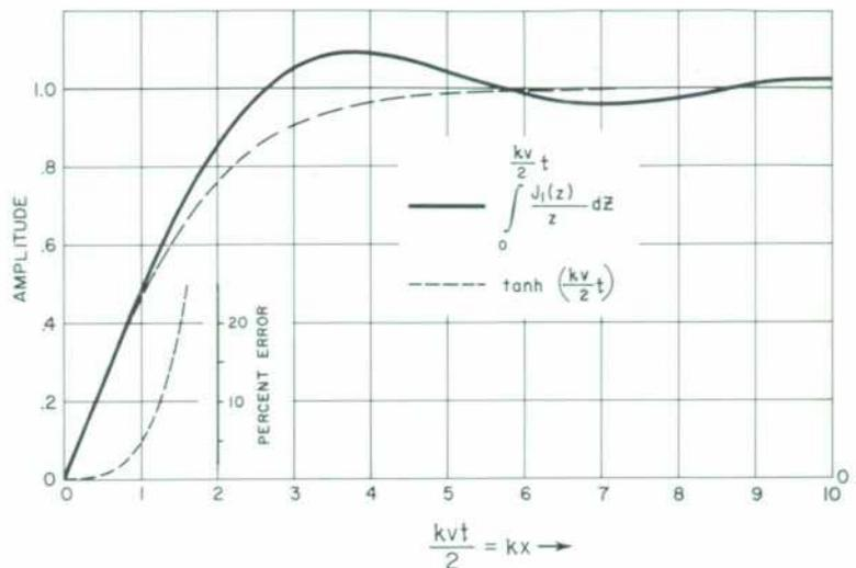
Fig. 11. The actual reflection from an infinite exponentially tapered line (solid), and the line impedance profile plotted on the vertical scale  $y = (Z - Z_0)/(Z + Z_0)$  (dashed curve). The error incurred from reading impedance off the solid curve is under 7% for  $Z/Z_0 < 3$ .
