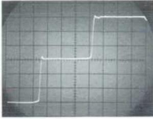
Fig. 13. Three feet of RG-9/U open circuited. Sweep speed 2.5 ns/division. The round trip delay is 3.8 divisions or 9.5 nanoseconds. The propagation velocity is thus 193 meters/microsecond or 64% of the velocity of light. The dielectric constant is therefore  $(1/64)^2$  or 2.4.
