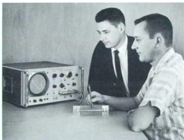
Fig. 1. Time domain reflectometer setup using -hp- Model 1415A plug-in unit with -hp- Model 140A Oscilloscope. Plug-in unit generates a fast step which is fed to external circuit. Energy reflected by discontinuities and impedance changes in external circuit returns to plug-in and is displayed on oscilloscope, permitting magnitude, sign and physical location of discontinuity to be read from scope face.
