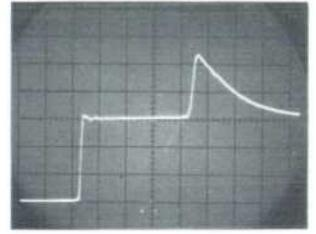
Fig. 16. Reflection from a lumped inductance of 330 nanohenries in series with a 50-ohm line. Sweep speed is 2.5 ns/cm. The time constant is  $L/2Z_0$  or 3.3 nanoseconds. The finite rise time of the step prevents the voltage from quite doubling.
