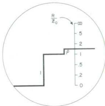
Fig. 4. After the reflection from a resistive termination the trace has the height  $1 + \rho = 2R/(R + Z_0)$ . This is the scale law of the simple ohmmeter shown in Fig. 3. Such a scale on the scope face permits impedance to be read directly.
