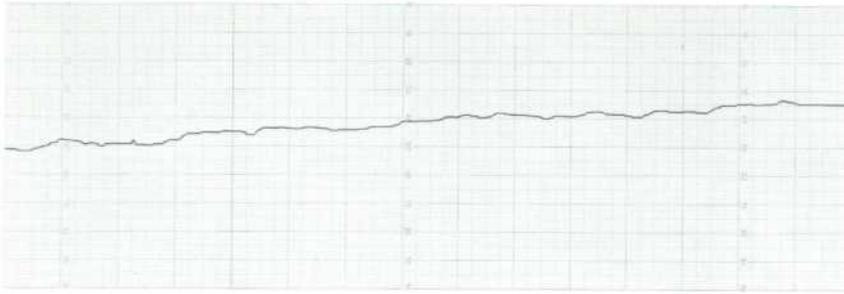
Fig. 4. High stability of Model 1400A 100  $\mu\text{v}/\text{cm}$  amplifier is shown by one-hour recording of dc drift. Major vertical divisions represent 0.1 mv referred to plug-in input, indicating drift of less than 0.2 mv/hour after warm-up.
