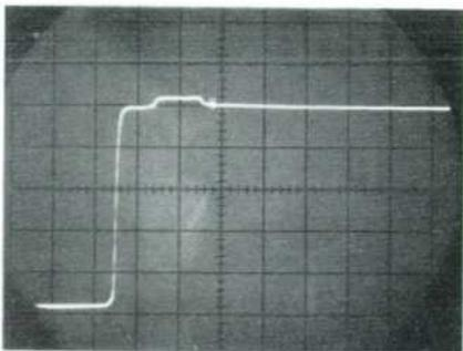
Fig. 3. Difference in cable impedances is shown by this oscillogram. Initial portion of step represents 3 ft of 50-ohm cable. Raised portion is caused by 5-ft cable that has 52-ohm impedance. Remaining portion of step represents 50-ohm cable termination.
