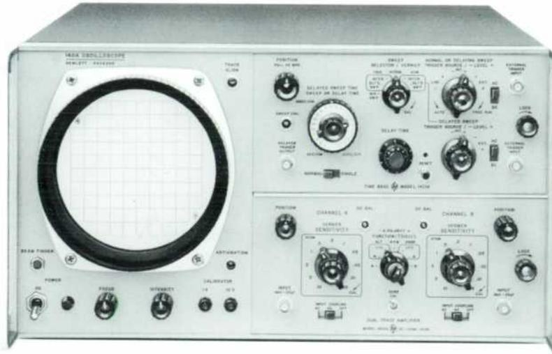
Fig. 1. For maximum flexibility, new -hp- Model 140A Oscilloscope has all deflection circuitry in plug-ins. Measurement range spans dc to 20 Mc and sensitivities to 10  $\mu\text{v}/\text{cm}$ .
