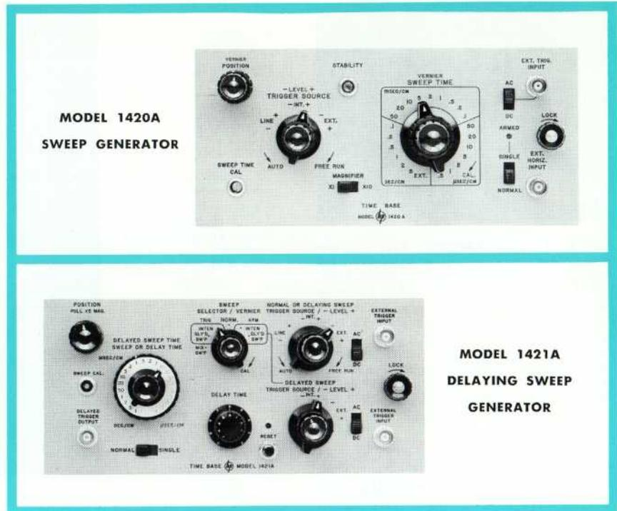
delay interval selected by front panel controls. In the delayed sweep *Arm* mode, the delayed sweep is started by the first trigger following the delay interval. Either *Trigger* or *Arm* modes likewise may be selected for the *Intensified* operation described earlier.
