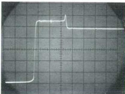
Fig. 2. Impedance mismatch between 50-ohm coaxial cable and 39-ohm termination is shown by oscillogram made with -hp- Model 140A oscilloscope and Model 1415A Time Domain Reflectometer plug-in. Sharp spike results from inductance of termination leads. Bright dot corresponds to setting of calibrated dial on delay control, permitting quick location of discontinuities. (Sweep speed: 4 nsec/cm)
