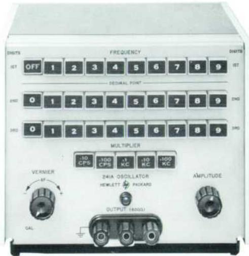
Fig. 3. Panel view of new *-hp-* Model 241A Push-Button Oscillator. Push-buttons permit selecting 4500 output frequencies from 10 cps to 1 megacycle (999 kc). Frequency vernier provides overlap between switch frequencies.
