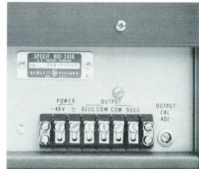
Fig. 2. Input and output terminal arrangement on instrument rear panel.
