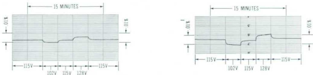
Fig. 8. Curves showing typical small effect of large line voltage changes on output frequency. Left curve measured on 1 kc output frequency, right curve at 100 kc.
