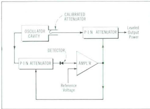
Fig. 3. Basic circuit arrangement of new hp-Model 8614A UHF Signal Generator.
