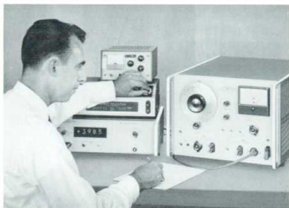
Fig. 1. Hewlett-Packard Model 4301A Variable Frequency Power Supply furnishes up to 250 volt-amperes at frequencies from 40 to 2000 cps. Output voltage is continuously adjustable from 0 to maximum of 130 or 260 volts. Unit also can serve as excellent line isolator.
