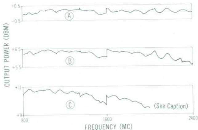
Fig. 6. Expanded-scale recordings showing typical leveled outputs obtainable at rated and above-rated ("B" and "C") leveled powers. Reduced frequency coverage ("C") occurs at higher powers, but usable range is still wide.
