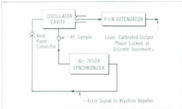
Fig. 12. Dymec 2650A Synchronizer can be used to obtain short-term stabilities of  $1/10^6$  from Generator at discrete frequencies.
