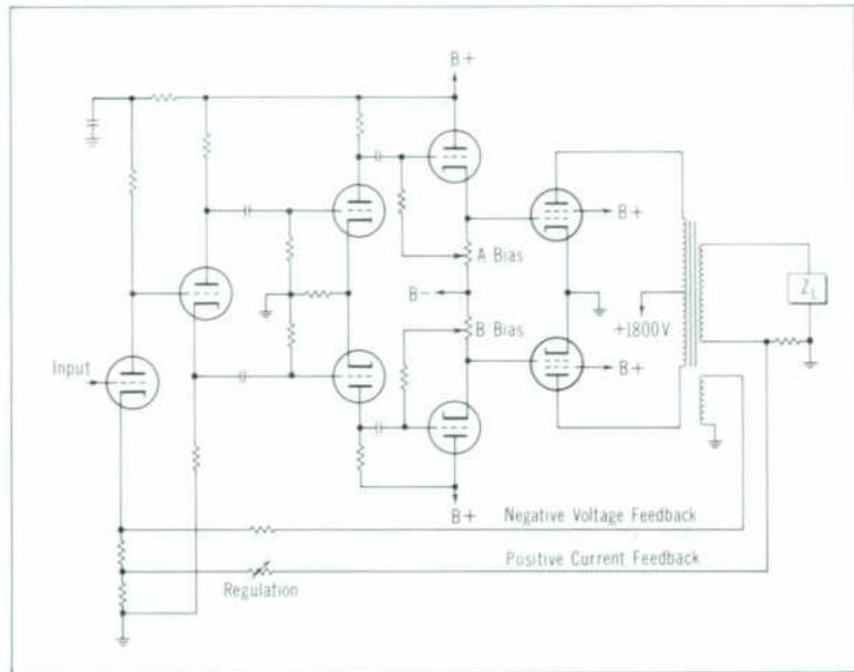
Fig. 4. Circuit diagram of 250 va power amplifier. Transformer output winding actually consists of two windings that may be switched from front panel for either series or parallel operation.
