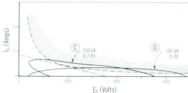
Fig. 8. Reactive load lines illustrate necessity for derating output power when instrument drives loads having power factors of less than 0.7.
