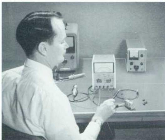
Fig. 1. New -hp- Model 410C Multi-Function Voltmeter has been designed as a general-purpose dc-measuring instrument which can also measure ac to 700 megacycles with detachable ac probe (shown at left of 410C in center). Instrument's high current sensitivity permits measuring small currents as in above photo, where diode leakage current of 1.6 nanoamperes is being measured.
