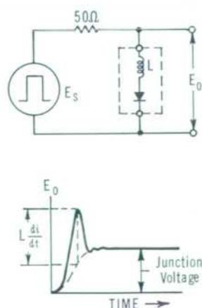
Fig. 6(b). Explanatory drawing for Fig. 6(a).
