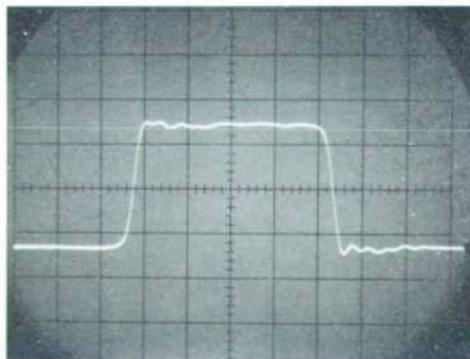
Fig. 2. Oscillogram showing typical quality of fast pulse provided by new generator. Width of pulse shown is 10 nanoseconds, rise time is less than 1 nanosecond, and overshoot less than 5%. Amplitude of pulse shown is 10 volts across external 50 ohms.
