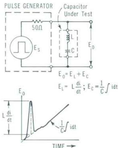
Fig. 1(b) (at right). Explanatory drawing for Fig. 1(a).
