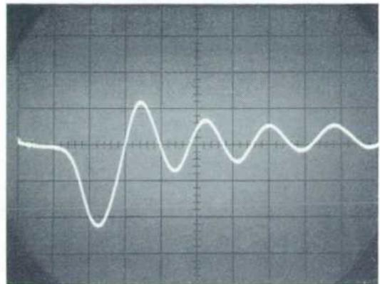
tance gives  $L = (50)^2 (2.5 \times 10^{-12}) = 6.25$  nanohenries/inch. One inch of this cable, with the far end shorted, was used to obtain the calibrating waveform shown in Fig. 2.
