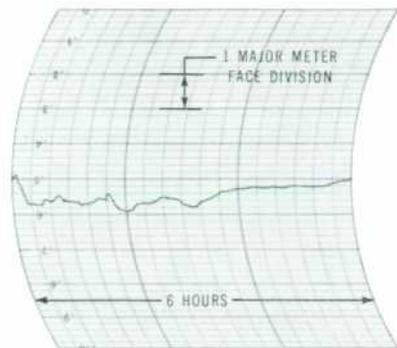
Fig. 5. Six-hour recording of room-condition zero-drift on most sensitive range of new power meter shows high stability achieved. This drift then becomes attenuated by range factor on higher ranges.
