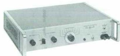
Since input data is stored and changes only when the input changes, accuracy of conversion is maintained at high sample rates. Specified accuracy is 0.5% full scale or better with a resolution of 0.1% full scale.
