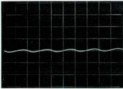
Fig. 7. Oscillograms demonstrating improvement in regulation obtainable at load by use of remote sensing feature of Model 722AR. Normally, remote sensing is used for improvement in dc regulation rather than ac which is shown here for clarity of illustration. Vertical scale is 50 mv/cm.
