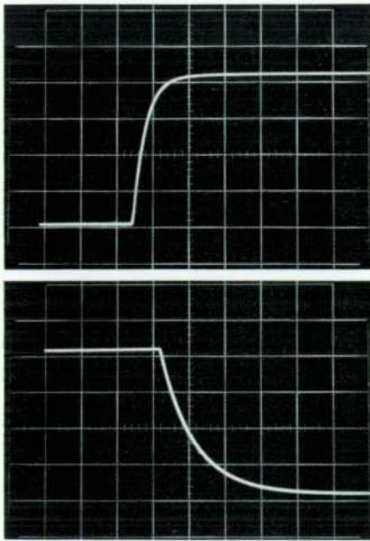
Fig. 9. Oscillograms of turn-on and turn-off characteristics of Model 723A power supply. Vertical scale is 10 v/cm; sweep time is 0.2 sec/cm.
