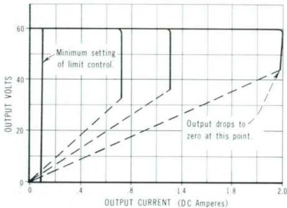
Fig. 3. Typical current-limiting characteristic of hp-Model 722AR for various settings of current-limit control. For large current overloads an electronic circuit turns off output voltage, as shown by dashed lines.
