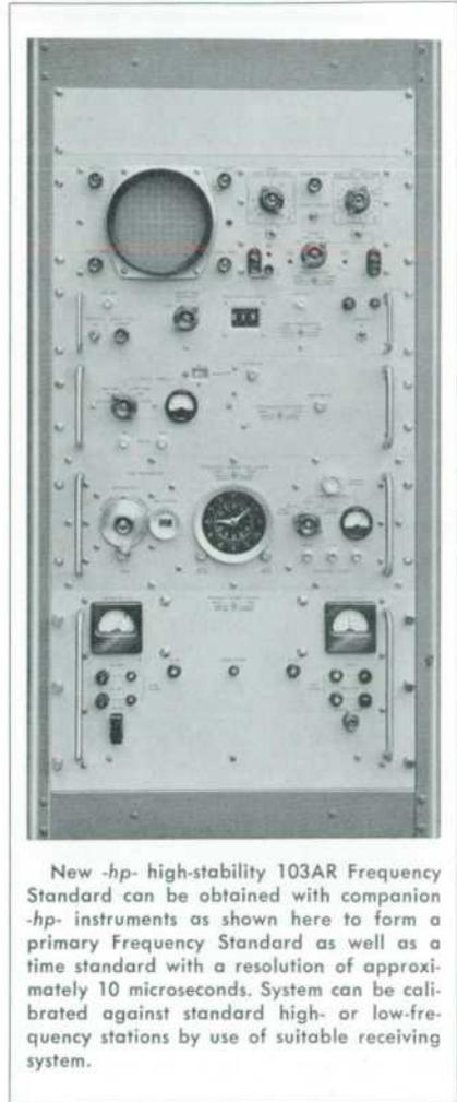
New -hp- high-stability 103AR Frequency Standard can be obtained with companion -hp- instruments as shown here to form a primary Frequency Standard as well as a time standard with a resolution of approximately 10 microseconds. System can be calibrated against standard high- or low-frequency stations by use of suitable receiving system.
