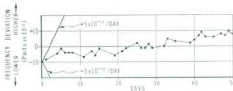
Fig. 2. Typical long-term stability performance of hp-103AR Frequency Standard after several-week aging period and under laboratory conditions. Solid  $5 \times 10^{-10}$ /day lines indicate rated performance of standard over  $0$ - $50^\circ\text{C}$  temperature range.
