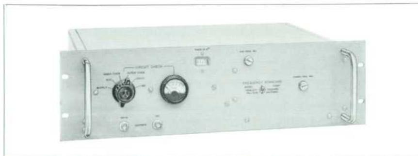
Fig. 4. Panel view of new *Frequency Standard*. Panel height is  $5\frac{1}{4}$ ". Output terminals are also provided on rear panel.
