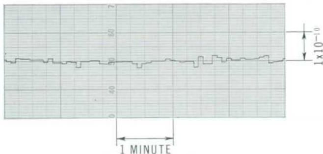
Fig. 9. Record showing 103AR output frequency as a function of large line voltage excursions when typical 103AR is operated from -hp- 724 Standby Power Supply. Vertical scale is  $10^{-11}$  per small division, time scale is 20 minutes per large division.
