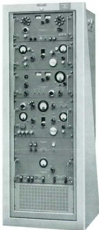
*Dymec signal simulator used for production tests of missile radar equipment.*
