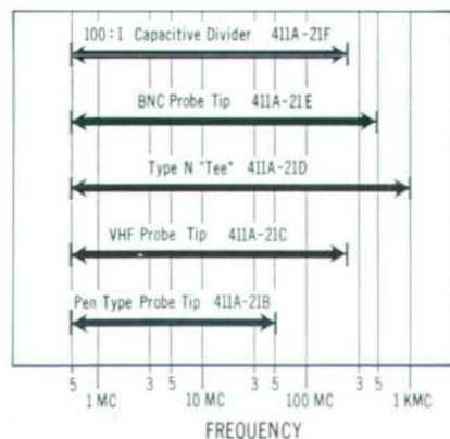
Fig. 9. Reference chart of frequency ratings for 411A accessories.
