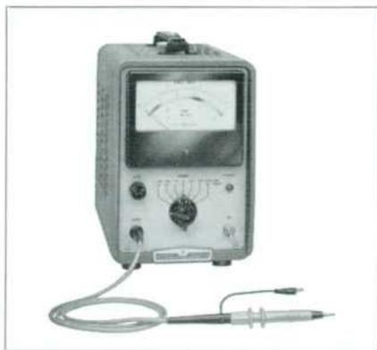
Fig. 3. -hp- Model 411A RF Millivoltmeter. Probe is arranged to accommodate many measurement conditions since basic probe tip with flange-operated alligator jaws as shown is removable; probe can then use various specially-designed accessories such as rf fittings for measurements in coax cables.
