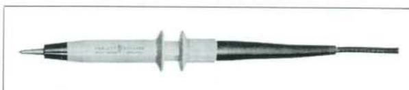
Fig. 19. Sync probe provided on oscilloscope.
