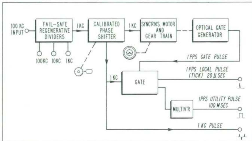
Fig. 7. Basic circuit arrangement of new Frequency Divider and Clock.
