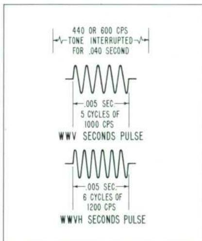
Fig. 3. Detail of seconds pulses transmitted by WWV and WWVH.
