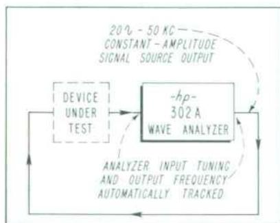
Fig. 5. Signal source output simplifies testing external circuits since analyzer input is tracked with this output. A measured frequency output is alternatively available to enable complicated spectra to be plotted with frequency counter.
