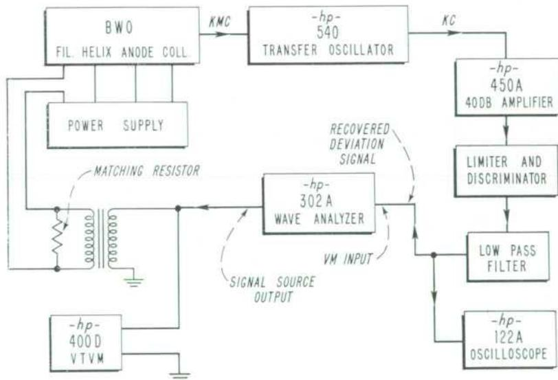
measured with the analyzer. With the coefficients of the tube elements thus established, a realistic basis is available for specifying power supply performance.
