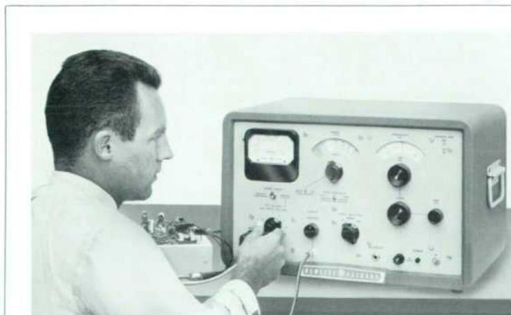
incorporates AFC circuit and linear tuning dial to simplify tuning. Voltage-measuring range extends below 10 microvolts. Instrument has sine wave output at dial frequency to facilitate transmission tests on external circuits.
