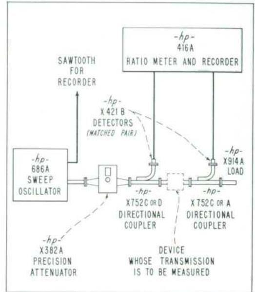
Fig. 3 (b) (at right). Equipment arrangement for measuring transmission characteristics in permanent-record form. If desired, wavemeters can be inserted as in Fig. 3 (a).
