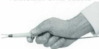
Tuning the capacity of the probe has also been made simple and requires no tools whatsoever. The probe capacity can be adjusted by loosening the finger-operated nut behind the rear flange. When this has been done, the rear flange can be rotated with respect to the rear part of the probe, thus adjusting the capacity. A convenient method of checking the capacity adjustment is to connect the probe to the square-wave calibrator voltage available on the oscilloscope panel.
