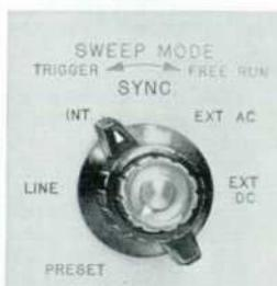
Fig. 8. Trigger Level and Slope controls (above) with Sync and Sweep Mode controls (below). When Sweep Mode control is in Preset position, sweep triggers automatically on most waveforms.
