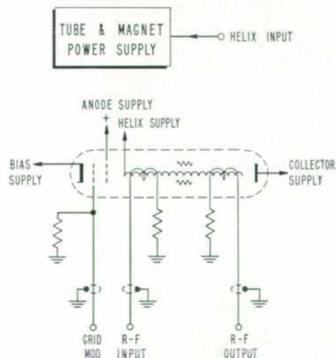
Fig. 2. Basic circuit arrangement of new amplifiers.
