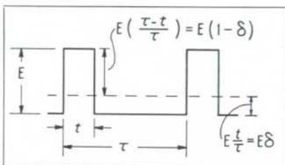
Fig. 8. Pulse waveform defining values used in text.
