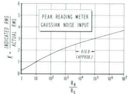
Fig. 10. Plot of correction factor for peak-reading meters when used to measure rms value of gaussian noise. Portion of curve applicable to *-bp-Model 410* is marked. Curve should be used only for rough estimating.
