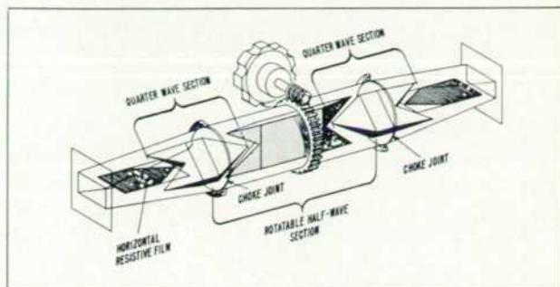
Fig. 2. Phantom view of *-hp-* Model X885A Phase Shifter showing relation of fixed  $90^\circ$  differential sections, the  $180^\circ$  rotatable section, and fixed end films which absorb horizontally-polarized output component.
