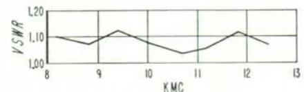
Fig. 5. Plot of typical VSWR of 8.2-12.4 kmc attenuator.
