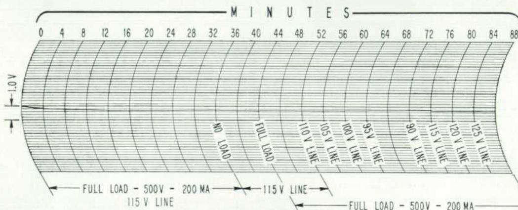
Fig. 2. Record made of main output voltage while 712B was subjected to wide changes in line voltage and output current.
