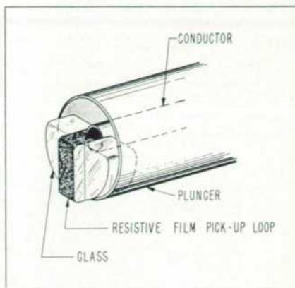
Fig. 5. Enlarged view of pick-up loops for attenuator and power monitor plungers.
