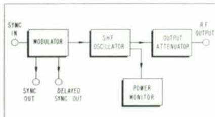
Fig. 2. Block diagram of Model 620A circuit arrangement.
