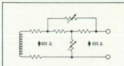
Fig. 7. Basic output circuit of *-hp-* 200CD.
