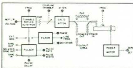
Fig. 1. Circuit block diagram of *-hp-* Model 624.
