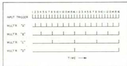
Figure 4. Schematic representation of operation of scale-of-16 circuit.
