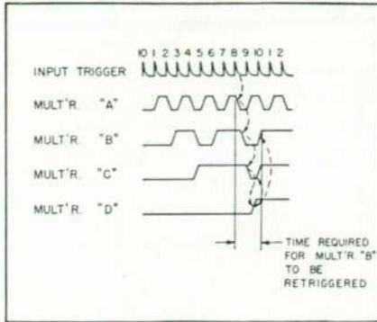
Figure 6. Delay in feedback circuit at high speeds.
