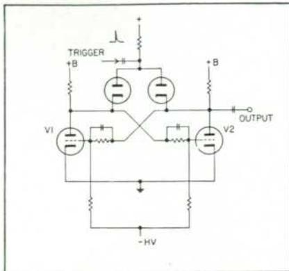
Figure 2. Basic bistable multivibrator circuit.
