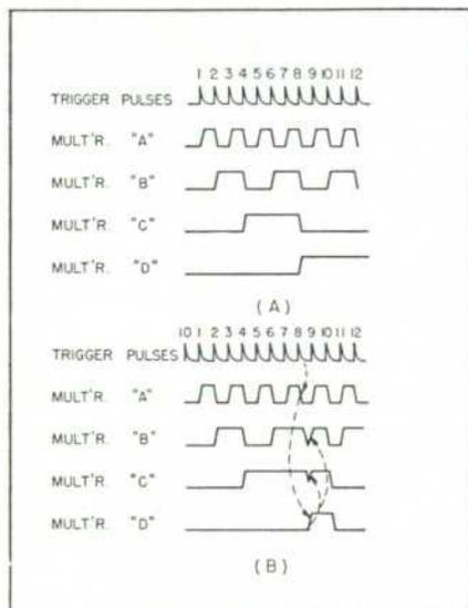
Figure 9. Operation of high-speed feedback circuit.
