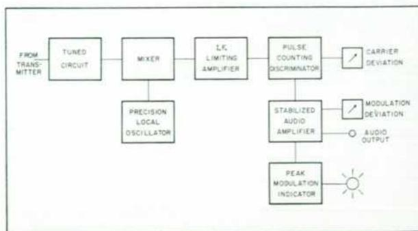
Figure 3. Block diagram of Model 337 monitor circuit.
