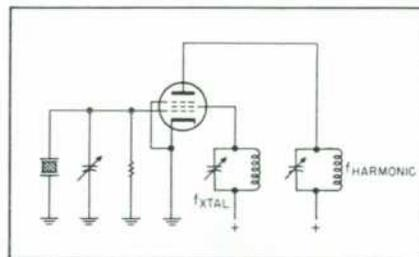
Figure 4. Basic circuit of reference oscillator.
