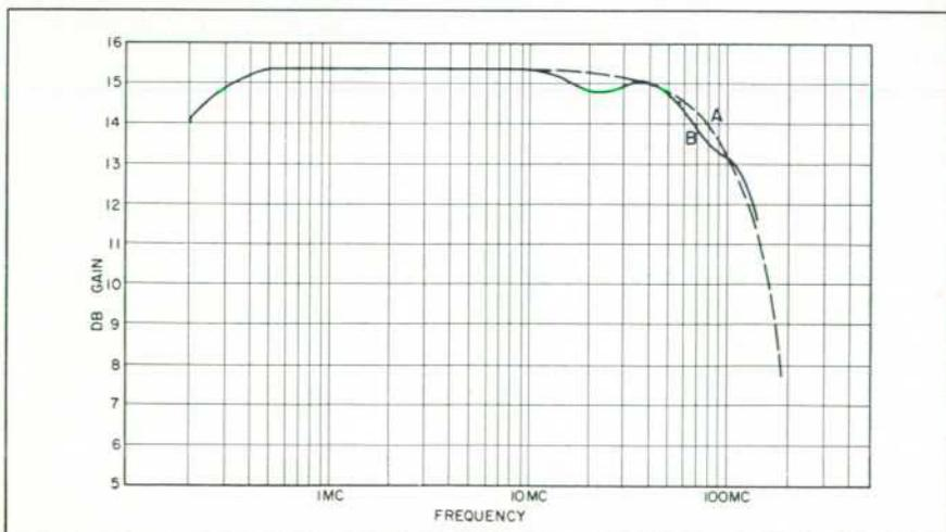
Figure 5. (a) Gaussian Response, (b) response of typical Model 460B amplifier.
