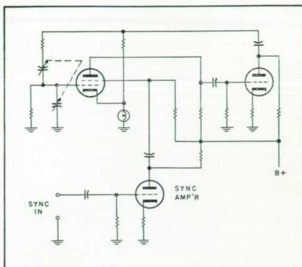
Figure 9. Circuit for Synchronization of Resistance-Capacity Oscillator
