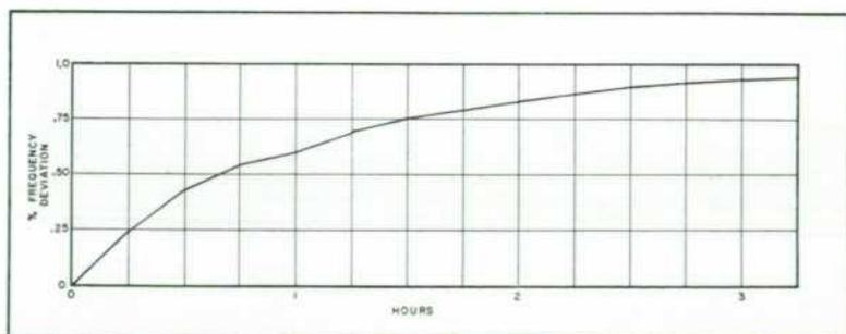
Figure 8. Short Time Stability Curve of Resistance-Capacity Oscillator
