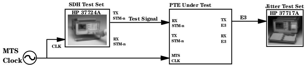
a) Synchronize Test Set to PTE by frequency locking Test Set's Transmitter to the MTS Clock used by PTE.
