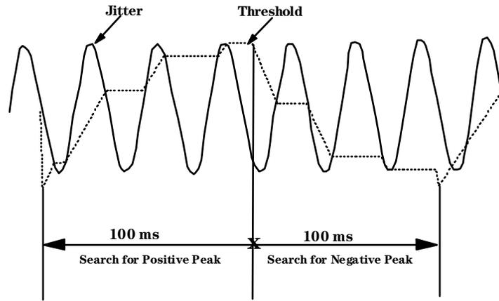
The peak-to-peak jitter during the 200 ms measurement interval is the difference between the positive peak in the first 100 ms, and the negative peak during the second 100 ms period. The maximum peak-to-peak jitter during a gating period is the largest value measured during one of the 200 ms measurement intervals.
