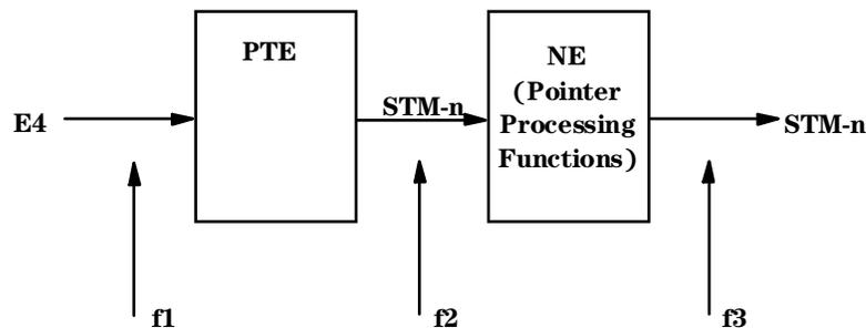
**Pulse Stuffing Rate controlled by f1 <-> f2**
