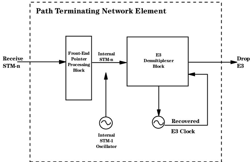
Figure 4: PTE test configuration.
