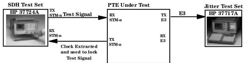
b) Synchronize Test Set to PTE by frequency locking Test Set's Transmitter to the Clock extracted from the SDH signal generated by the PTE.
