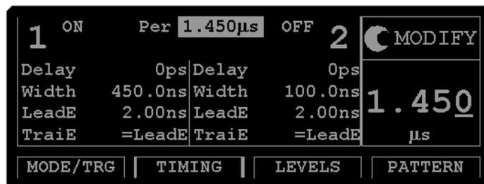
In order to get the 2.0 ms delay, we need to add leading zeros to the 18 bit pattern (the 81110A will not allow us to ask for more than 1.37 ms delay). With the RZ pulses set at 1.45 ms period we need 1,379 leading zeros. That will give us 1,999.55 ms of delay.
