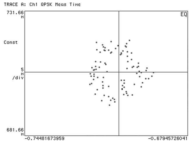
I/Q quadrature errors result in a tipped or skewed constellation (**Figure 21**). Quadrature errors are caused by a phase shift other than  $90^\circ$  between the I and Q paths. Different group delays in the baseband I and Q filters also create quadrature errors. This distortion of the constellation increases the possibility of errors in the interpretation of the received symbols and will increase the Error Vector Magnitude (EVM).
