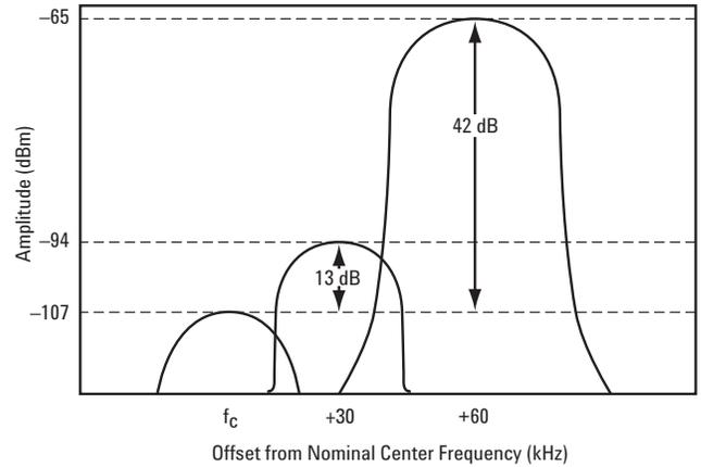
**Figure 18. PDC Adjacent and Alternate Channel Selectivity Spectrum**
