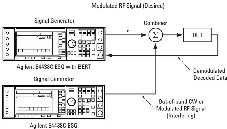
Figure 12. Intermodulation Products
