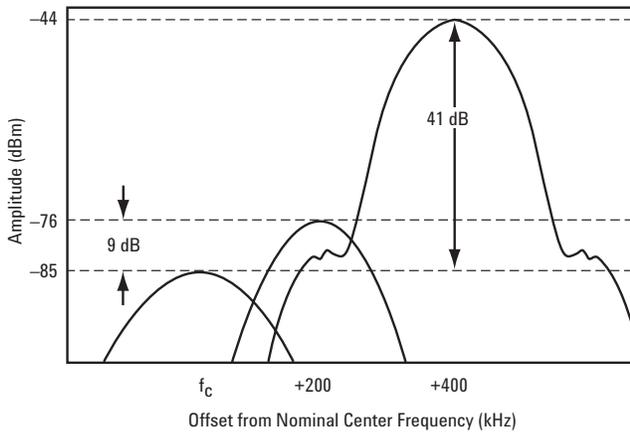
**Figure 17. NADC Adjacent and Alternate Channel Selectivity Spectrum**
