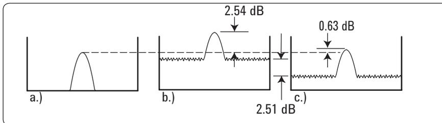
**Figure 18.** Log averaging improves the measurement of CW signals when their amplitude is near that of the noise. (a) shows a noise-free signal. (b) shows an averaged trace with power-scale averaging and noise power 1 dB below signal power; the noise-induced error is 2.5 dB. (c) shows the effect with log-scale averaging—the noise falls 2.5 dB and the noise-induced error falls to only 0.6 dB.
