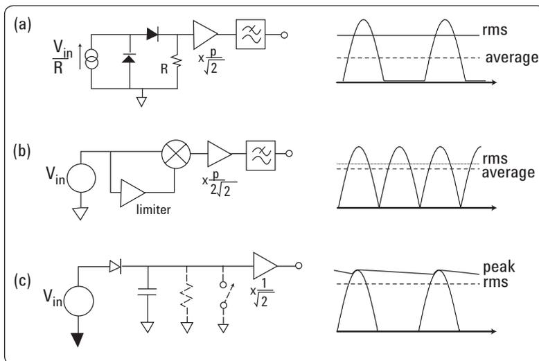
**Figure 9.** Detectors: a) half-wave, b) full-wave implemented as a “product detector,” c) peak. Practical implementations usually have their gain terms implemented elsewhere, and implement buffering after the filters that remove the residual IF carrier and harmonics. The peak detector must be cleared; leakage through a resistor or a switch with appropriate timing are possible clearing mechanisms.
