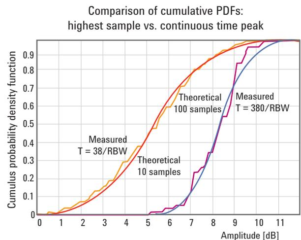
**Figure 16. Setting  $N$  a factor of 3.8 below the product of the observation time and the RBW gives good agreement between experiments with continuous time systems and theory for independent samples in this CDF plot.**
