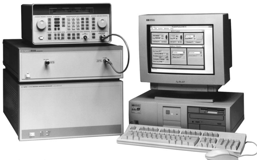
Figure 2. Multi-format communications signal simulator
