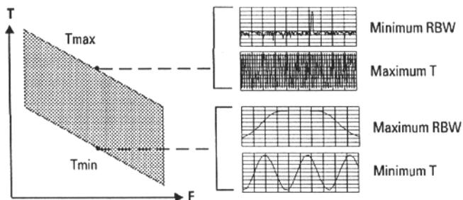
**Figure 7. Time and frequency resolution tradeoffs within the Agilent 89400 operating region**
