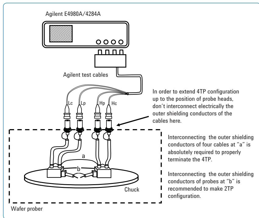
Figure 2. Cable extension and prober connection in four-terminal pair (4TP) configuration
