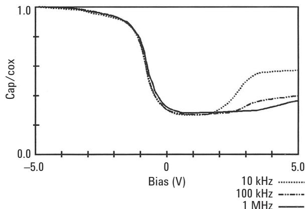
Figure 1. Multi-frequency C-V characteristics of a semiconductor
