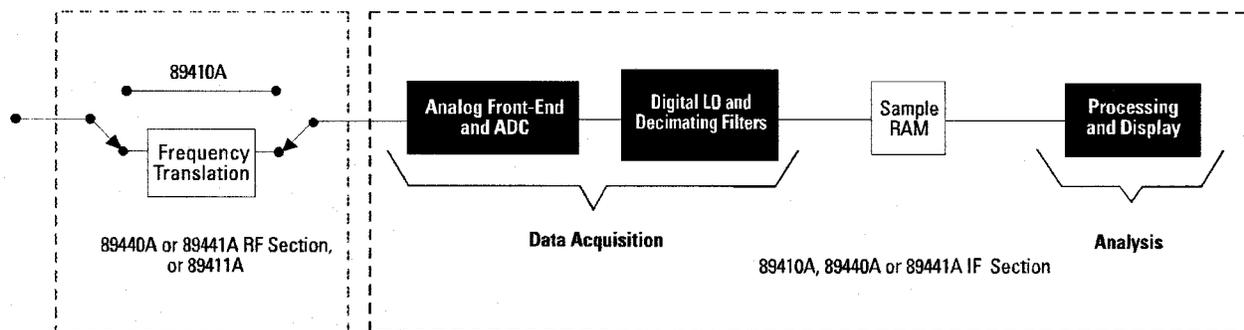
Figure 1. Simplified block diagram showing basic signal flow in the Agilent 89400 Series VSAs
