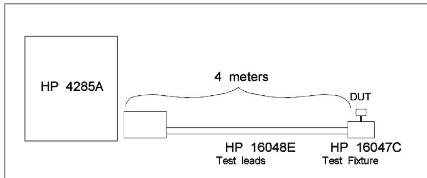
Figure 3. Cable Extension Using an HP 16048E (4m)
