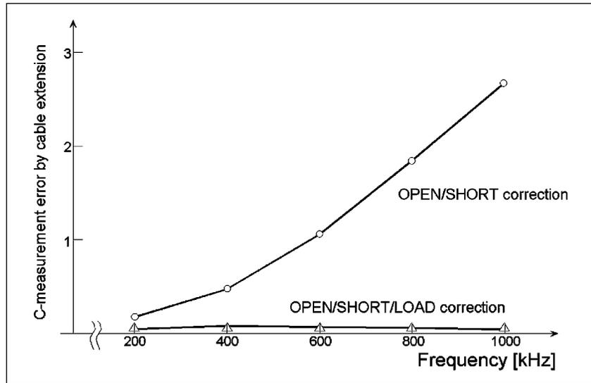
Figure 4. Comparison Between OPEN/SHORT Correction and OPEN/SHORT/LOAD Correction
