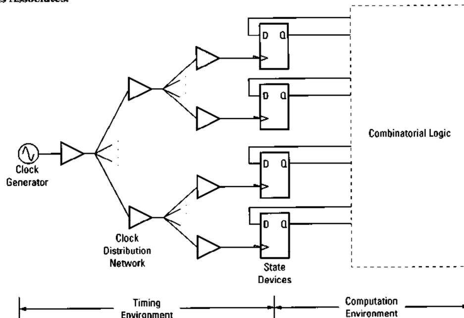
Figure 1. Timing Environment of a Digital System
